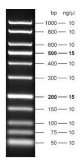
5µl loaded onto 1.8% agarose
